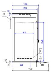
Electrical inlet (power) ΕI Refrigerant Outlet RO
